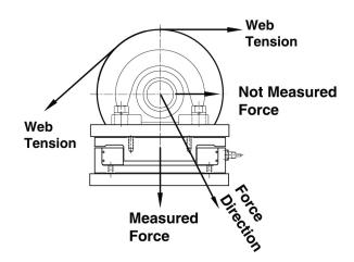
The BTV series, used in metal processing lines and other hostile industrial applications, accurately and reliably measure strip tension, and are designed to mount directly under the roll bearing pillow blocks.
